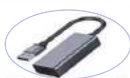
AIR-8156C 2500Mbps Chipset Realtek RTL8156 USB 3.0
